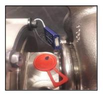
The seal number is the one associated to the turbo number as entered by its technical partner during original assembly or overhaul of it.
